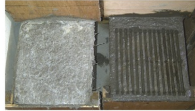
FIGURE 1: Difference of substrate surface conditions between being as-placed and grooved with 6 mm of roughness amplitude.
